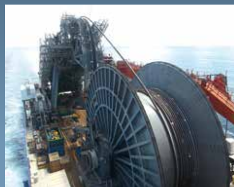
400 Te reel lay versatile system for rigid and flexible lay operations
