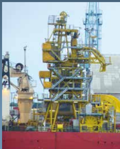
VLS the 7 th generation 135 Te Vertical-lay System
